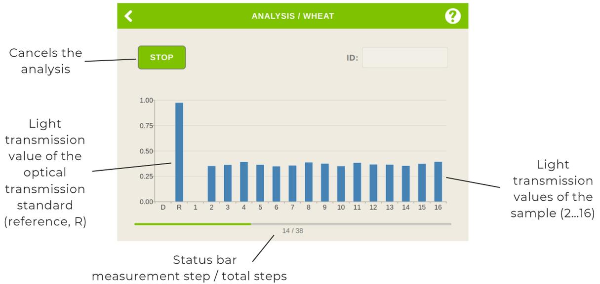
At the end of the measurement the results are displayed on the screen:
