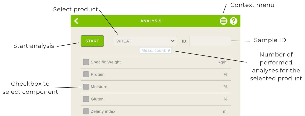
Components can be turned off by unchecking the checkbox:
